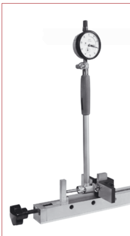
Orfeo con appoggio alesamento Orfeo with bore gauge support
